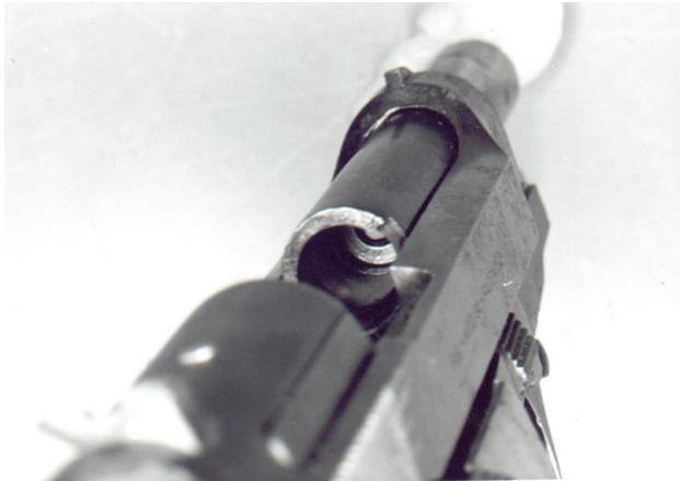
*Fig. 6&7 – A 7.65x17mm cartridge loaded into a Beretta's, model 84, chamber.
