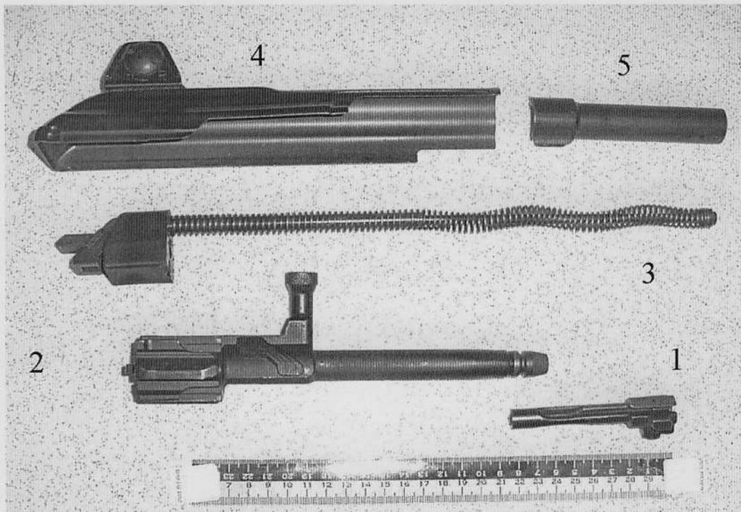
**Figure 4 – internal parts of the MAGAL**
